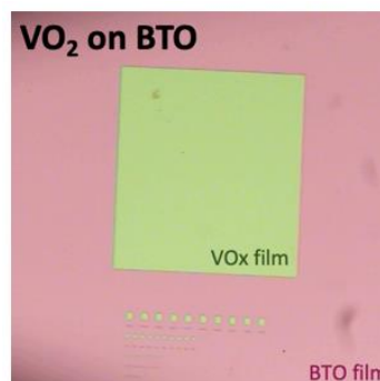
VO 2 film deposited on a BTO layer. left) optical microscope image, right) metal-to-insulator transition in VO 2 .
